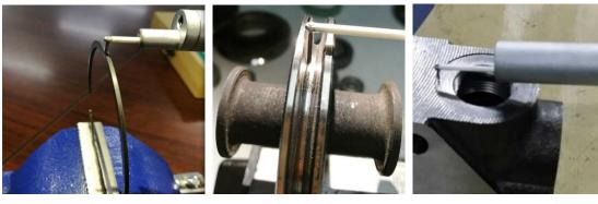
Narrow Ring Measurement Narrow Groove Measurement
