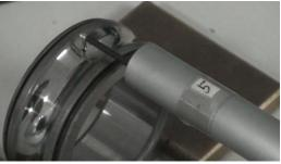
**External Raceway Measurement**
