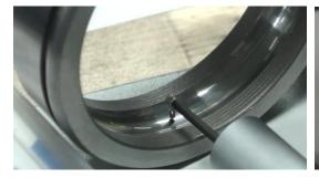
**Inner Raceway Measurement**
