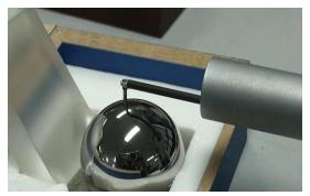
**Convex Spherical Measurement**
