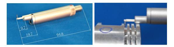
The surface measurement is not limited to roughness parameters. In the measurement of the scratches, the pickup is expected to rotate 90 degrees and skips along the arc. TIME®3231, with high resolutions and good straightness, achieves the breakthrough to access the profile information of small scratches.
