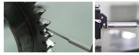
TIME S233 Pickup for Deep Groove (10 mm)
