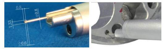
TIME S232 can also be applied for long and narrow spaces such as narrow tooth surface and grooves in piston ring.
